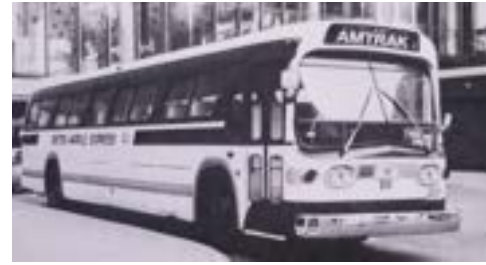
Service from Penn Station and Grand Central Station Is provided by a GM S8M-5304A in New York City.
